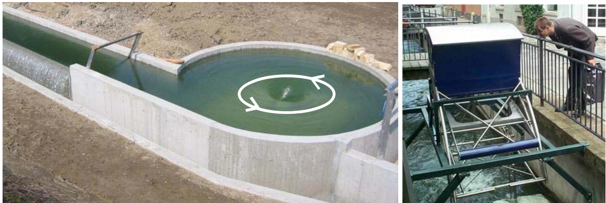
Fig. 9: (a) Gravitational Vortex Converter , side view of vortex, Zotlöterer (2006) and (b) photo of Aniprop , a stroke wing power generator, Aniprop (2006)
